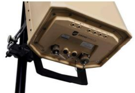
Interface panel includes system and frequency status LED indicators
