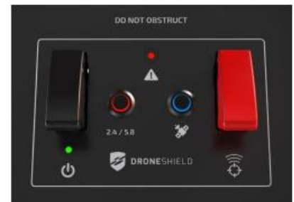
Simple control panel for frequency selection, standby and activation
